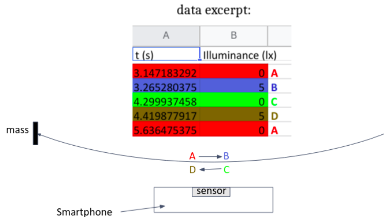
Fig.1. An excerpt of the raw data collected by the smartphone and their interpretation in relation to the motion of the pendulum.
