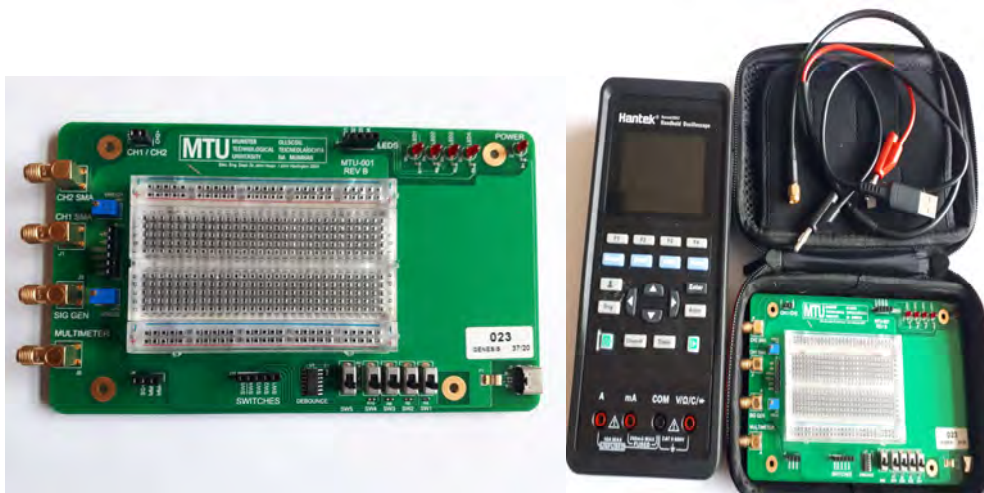
Fig. 2. HELP kit V1.0 laboratory board and board in carry case with Hantek 2D42
