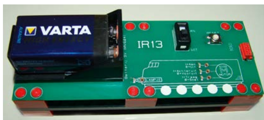
Fig. 3: picture of the IR13 emulator board. The train control part looks the same as on the real train with LEDs emulating the train behavior.
