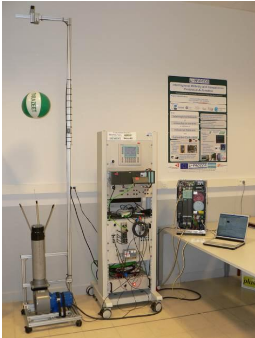
Fig. 3. Demonstrator beach ball levitation (developed by KU Leuven – Campus Ghent)
