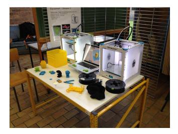
Figure 6: Ultimaker 3D printers of FabLab (University of Mons)
