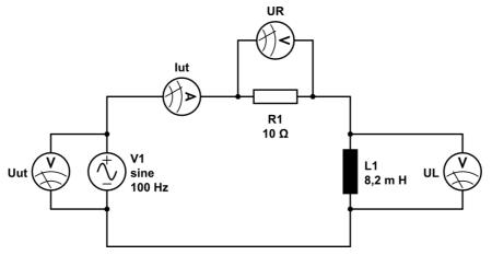
*Fig.* 3. An experiment in the first lab to investigate the validity of Kirchoff's voltage law. The output voltage  $u_{out}(t)$ , current  $i_{out}(t)$ , the resistor voltage  $u_{R}(t)$ , and the inductor voltage  $u_{L}(t)$  is measured by the interface and the results displayed on the computer screen (see *Fig. 4*). The interface generates a sinusoidal output voltage  $u_{out}(t)$  with a frequency of 100 Hz and amplitude of 2 V.
