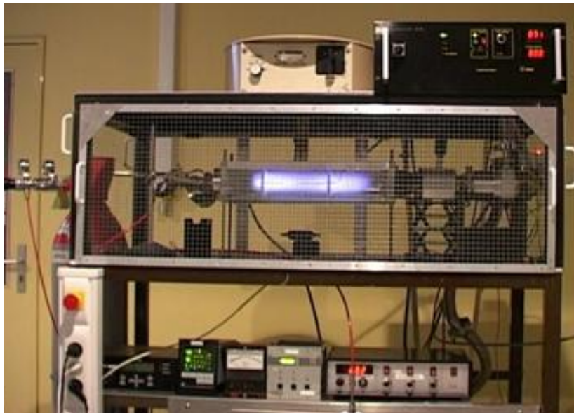
Fig 3: Picture of the experimental setup used for optical emission spectroscopy of an RF discharge in H 2 /Ar plasma.
