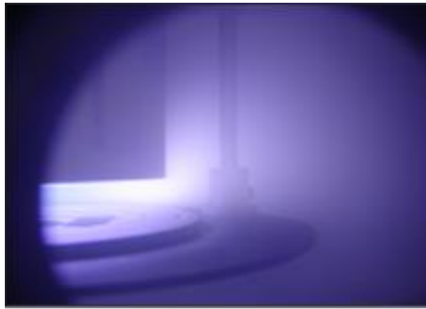
Fig. 5: Plasma deposition process by cathodic sputtering.
